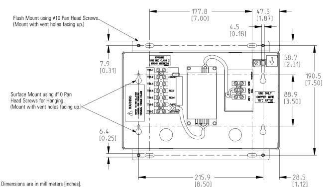
Figure 5-13. Relay Interface Module II Dimensions
